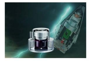
In the center of the battery case a glass ampoule filled with electrolyte (SOCI<sub>2</sub>) is located, which is broken by a special an application specific release mechanism, depending on the respective system acceleration.
